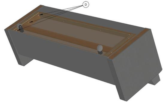
**D:** Using a ratchet and 7/16" socket, unscrew the six 3 1/4" long bolts that secures the Cross-Member Assembly to the Upper Deck. This Cross-Member Assembly along with the Lower Deck can now be separated from the Upper Deck, and set to one side.
