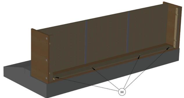
**M:** If the sleeper has an optional Back, with the aid of an assistant, lay the sleeper on its back and, with a knife, slice the fabric along the seam between the Back and the Upper Deck. Next remove the 4 Philips screws which attaches the Back to the Upper Deck. Now slide the Back up slightly, and then pull it away from the Upper Deck so as to free the metal clips securing the Back to the Upper Deck. Remove the metal clips with the Philips screwdriver.
