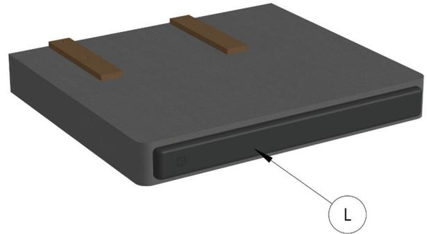
**L:** If the End Frames have optional arm caps, use a large flat blade screwdriver or a flat pry bar, to pry off the arm caps. Unscrew the threaded rods from the arm caps.
