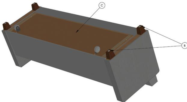
**B:** Using the Robertson screwdriver, remove the wood screws securing the four wood legs or the optional casters from the sleeper. Next, using a screwdriver pry the nylon glides off of the wood legs.
