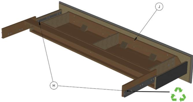
**H:** Now extend the Lower Deck and the Cross-Member Assembly apart from each other in order to gain access to the 12 Robertson screws securing the metal slides. Once the slides are removed the two assemblies will be separate from each other.
