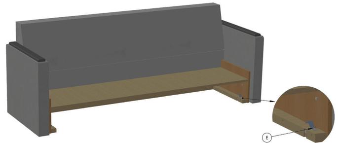
**E:** Remove the metal spring clips from the two hardwood spacers.
